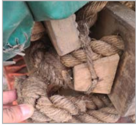
Embarkation ladders (Port and Star board) side rope wasted [Not properly maintained]
