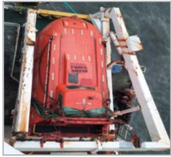
life boat found not operational [Inoperative]
