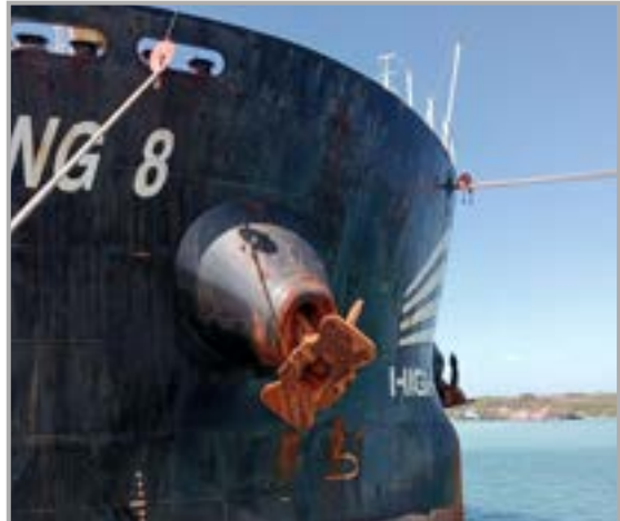
The Sea Anchor is much corroded [corroded]
