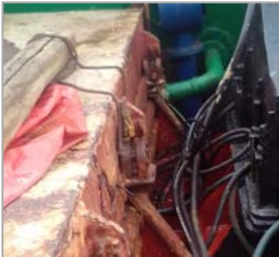
Hatch cover cleats not properly secured
